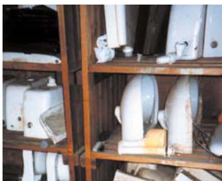
Figure 40 Asbestos-reinforced toilet cistern
