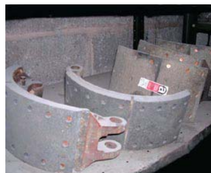
Figure 41 Asbestos brake linings for quarry vehicles
