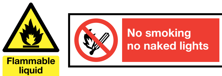
Figure 3 Example of warning and prohibition signs with supplementary text used at entry points to flammable liquid facilities
