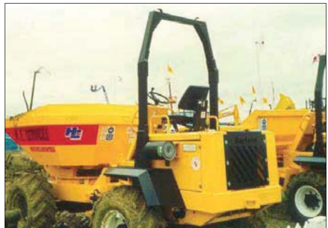
Figure 21 Rollover protective structure (ROPS)
