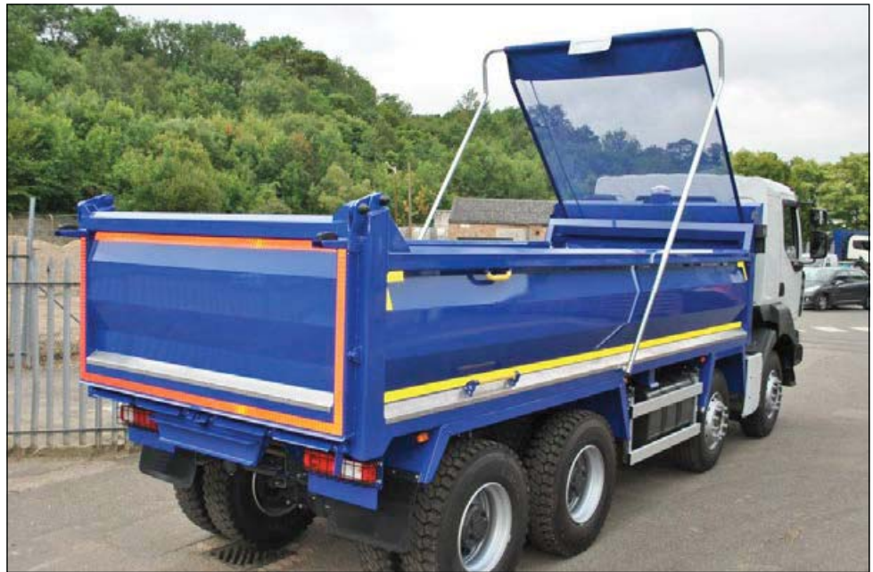
Figure 20 Front-to-rear sheeting system
