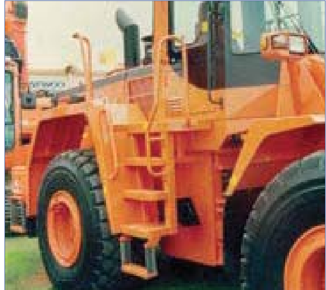
Figure 18 Access to vehicles – steps and handrails
