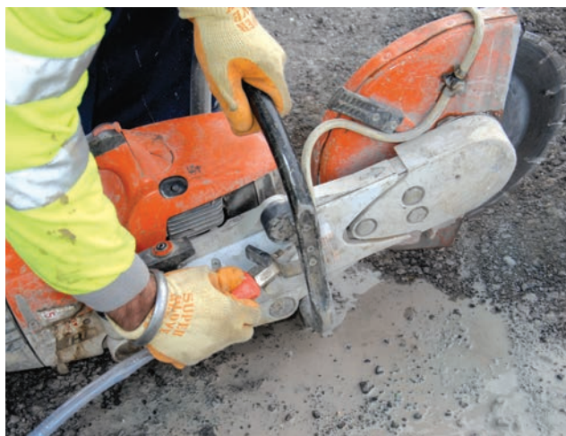
Figure 3 Water suppression on a cut-off saw
