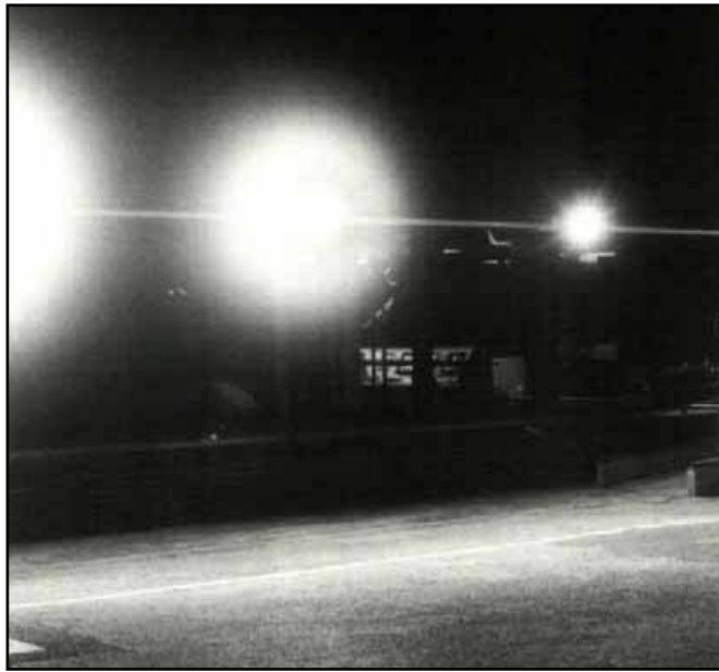
Figure 1 Disability glare from a light fitting
