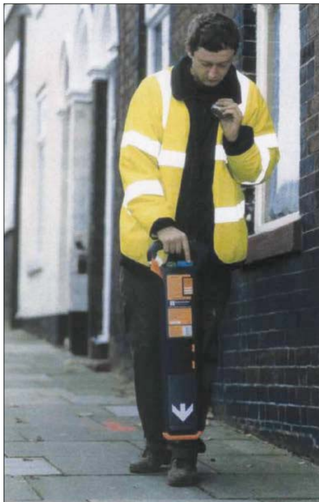
Figure 1 Using a cable locator
