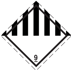
Figure 7.21 CDG hazard placard
