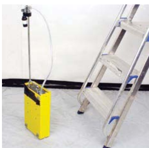
Figure 7.27 Air sampling during clearance
