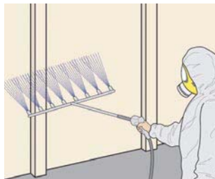
Figure 7.14 Multi-point spray system
