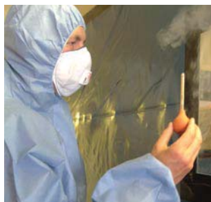
Figure 2.3 Supervisory licence holder checking the integrity of an enclosure
