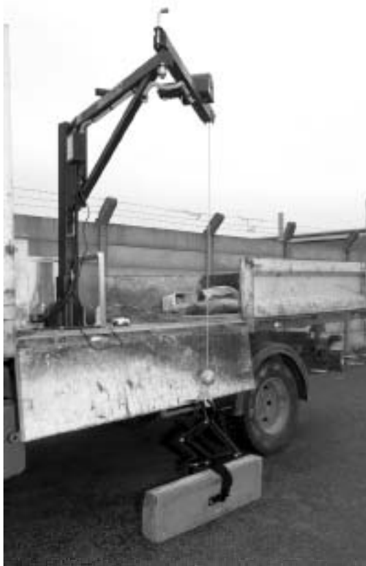
Figure 2 Vehicle-mounted crane and mechanical grab
