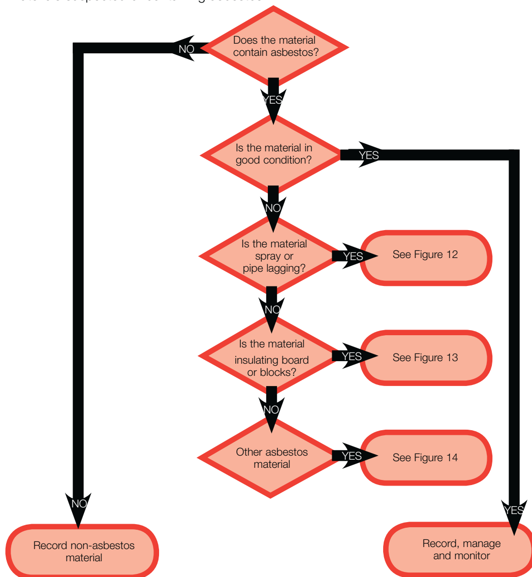
Figure 11 Materials suspected of containing asbestos
