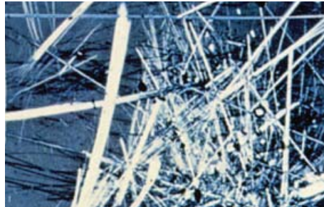
Figure 4 Asbestos fibres viewed down a microscope
