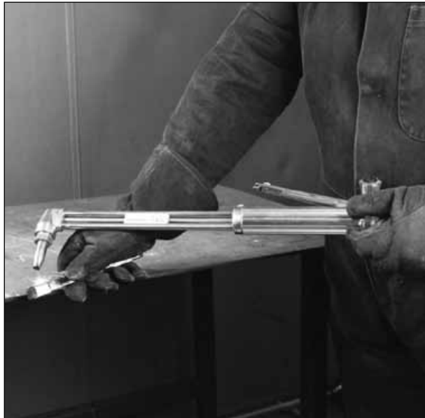
Figure 11 Lighting a blowpipe with a spark lighter
