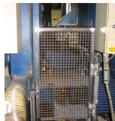
Figure 6 Older mechanically-fed six-in-line horizontal band saws with retrofitted interlocked hinged gate between machines
