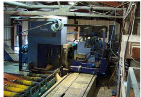
Figure 8 A reciprocating carriage log band saw – feed on to carriage and carriage approach to band saw
