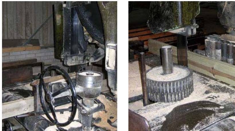
Figure 3 Stand-alone band saw with manual feed and optional power feed without guard fitted
