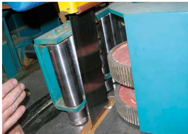
Figure 10 Single-cut band re-saw – details of feed rollers
