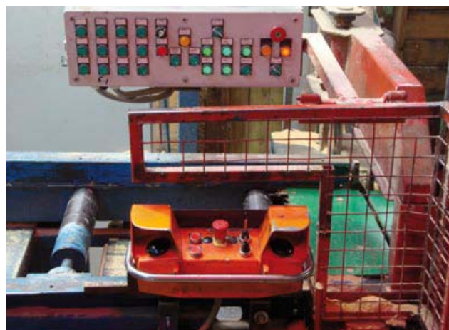
Figure 18 Semi-automatic rise and fall cross-cut saw with two-hand control
