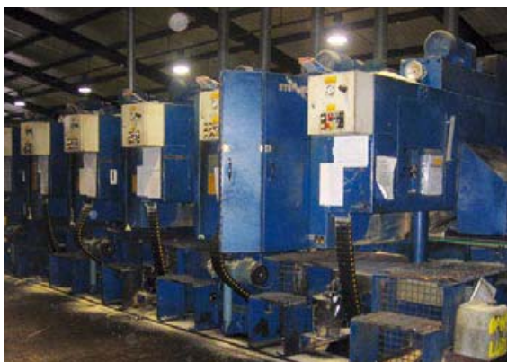
Figure 6 Older mechanically-fed six-in-line horizontal band saws with retrofitted interlocked hinged gate between machines
