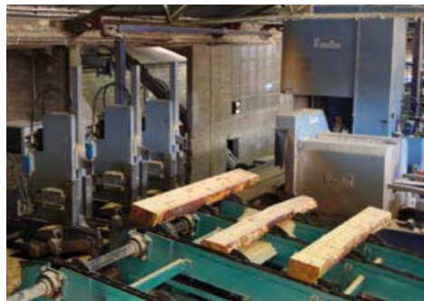
Figure 8 A reciprocating carriage log band saw – feed on to carriage and carriage approach to band saw
