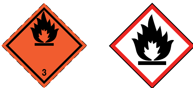
Figure 3 Examples of flammable liquid packaging labels
