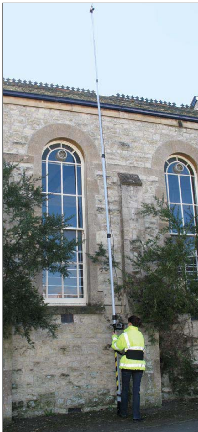
Figure 11 Remote inspection mast with hand-held light-weight CCTV system (Image courtesy of Survey Support Ltd)
