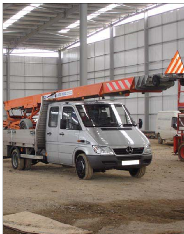
Figure 40(a) Mechanical handling of large roof sheets (Images courtesy of Advisory Committee on Roofsafety), see also Figures 5(a) and 5(b)
