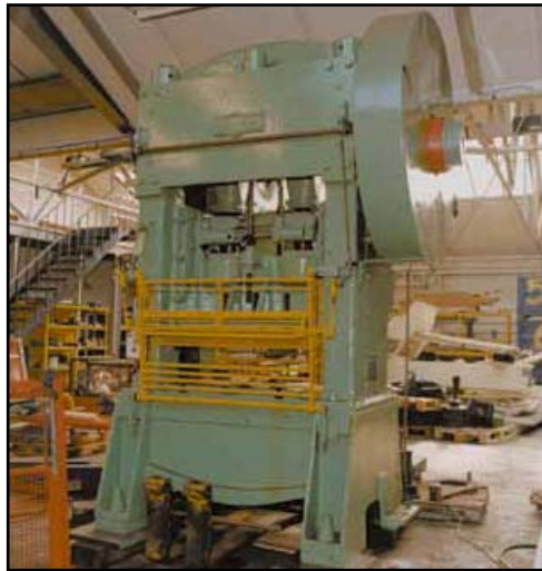
Typical interlocked guard
