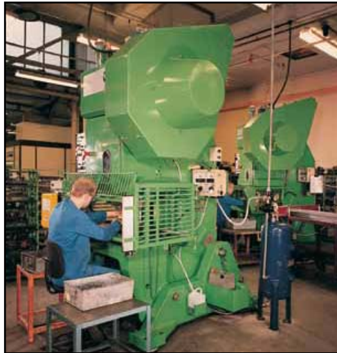
Open-fronted power press with light curtain
