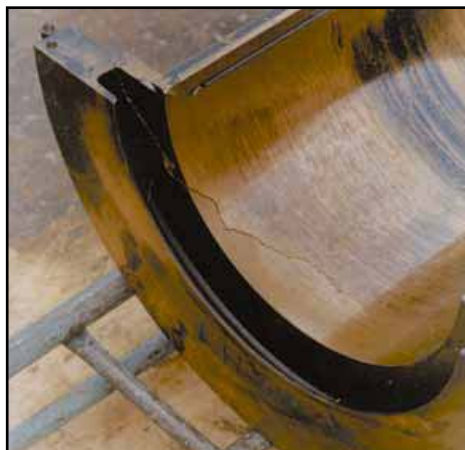
Severely cracked bearing
