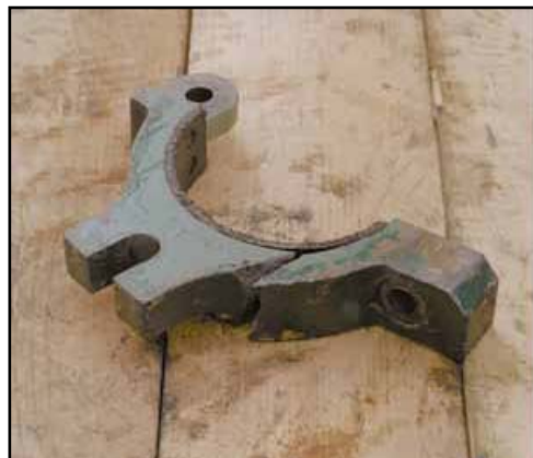
Cracked brake shoe
