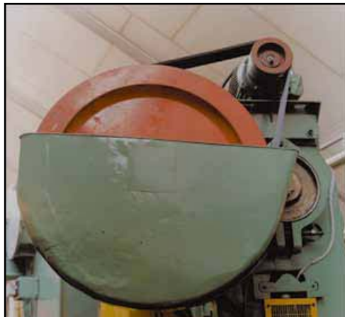
Flywheels need to be removed periodically
