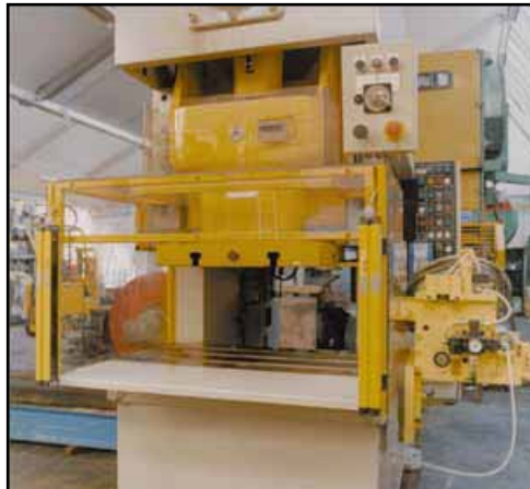
Power press fitted with a light curtain
